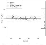
This graph shows plots of the error  $(SpO_2 - SaO_2)$ by SaO<sub>2</sub> using the 9550 with a linear regression fit and upper 95% and lower 95% limits of agreement. Each sample data point is identified by subject from a clinical study in non-motion conditions.
