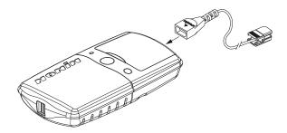
Figure 4: Connecting the Sensor
