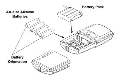
Figure 3: Installing Batteries
